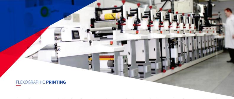
Flexographic printing uses flexible photopolymer printing plates wrapped around rotating cylinders on a web press. The inked plates have a slightly raised image and rotate at high speeds to transfer the substrate.
